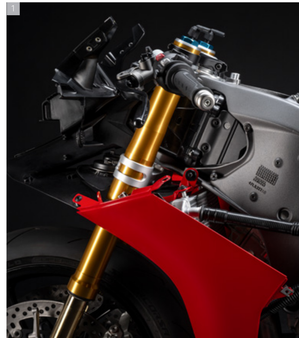
1 Öhlins NPX 25/30 (SV) S-EC 3.0 pressurized 43 mm fully adjustable fork with TiN treatment. Electronic compression and rebound damping adjustment with Öhlins Smart EC 3.0 event-based mode
